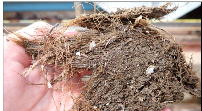
Hydrooids – a challenging trash rack biofouler
